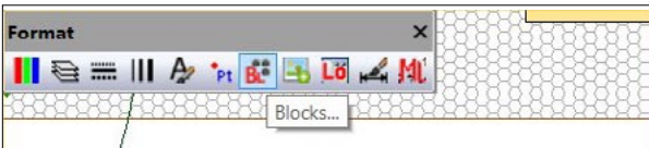
The BLOCKS command is used to insert symbols.
