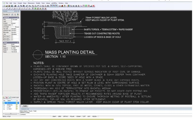
Here the text under the heading NOTES is applied with the MTEXT command.
