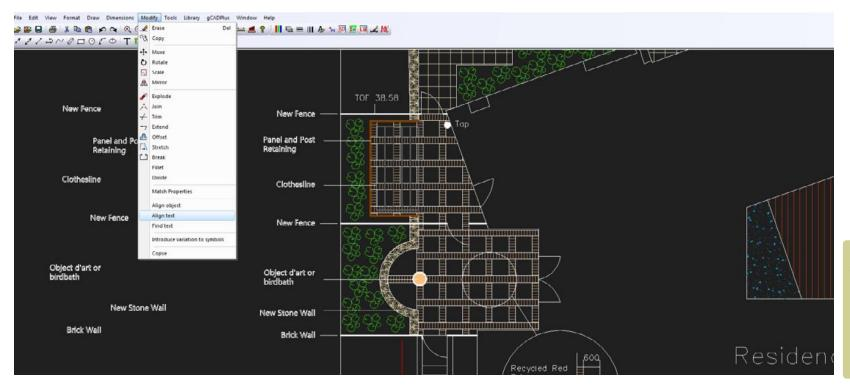
Here the align text tool is used to right justify a series of text objects that were originally arranged as show on the left of screen.
