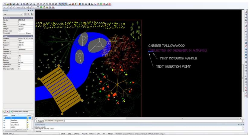
Single-line text showing insertion point and rotation handle. The properties box enables changes to be made to alignment - left, right, center justified etc.
