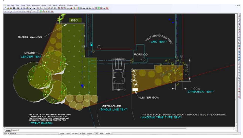
Single line text, multi line text, Windows True Type text and arc text are all used in this drawing. Some lettering styles here use CAD fonts, others use Windows fonts.
