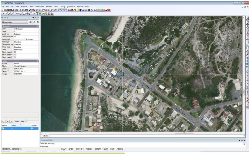
Here a very large, high-resolution aerial photograph of part of the South Australian coastline loads and displays in seconds in gCADPlus and displays the correct MGA coordinates. The file is 1.5 Gig in size!
